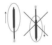
The piston of the gasspring must be at the top
